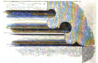
Cornice, or Wall Plate of Roof, Beckley, Oxfordshire, c. 1330.
